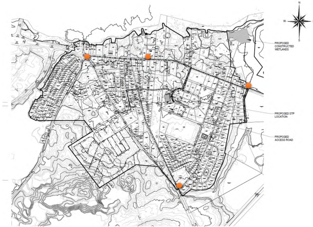
Figure 2 - Alternative Pumping Station Locations (in Orange)
