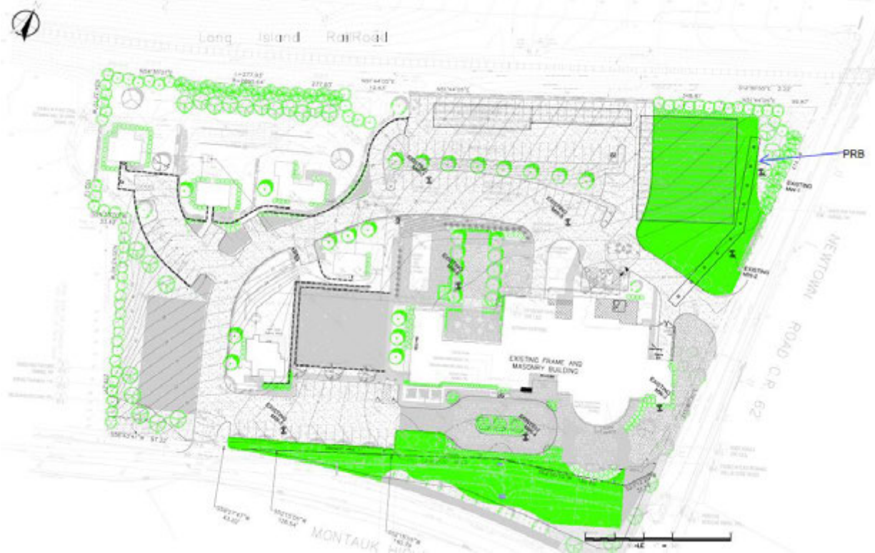
Figure 5-2 CPI Drainfield and PRB Layout
