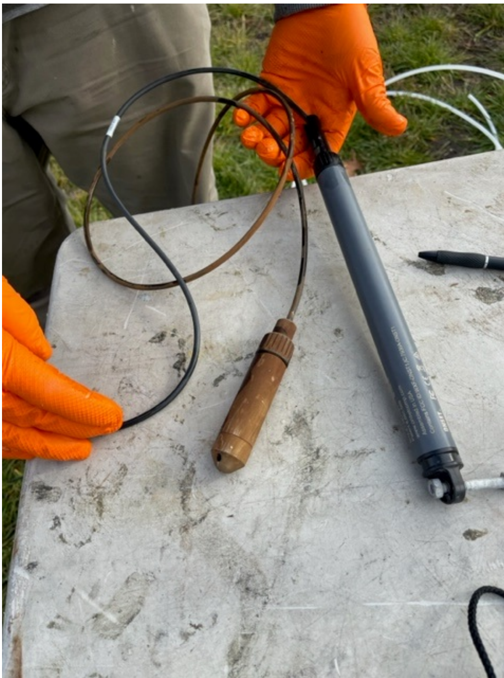
Figure 2-5 Well UG-3 GW Elevation Monitoring Device Iron Staining
