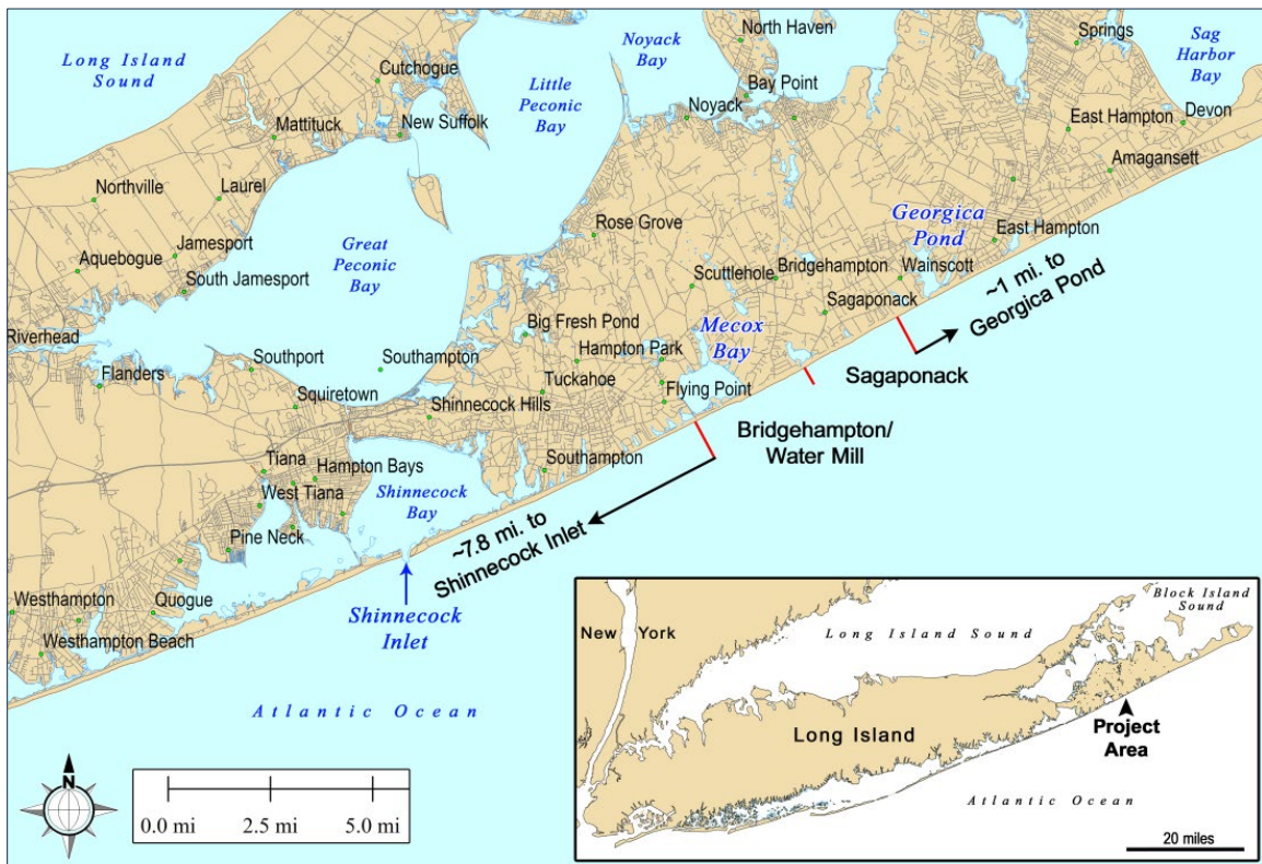
FIGURE A. Project location map showing the Sagaponack–Bridgehampton–Water Mill beach nourishment project area situated along the mainland bluff shoreline of eastern Long Island. Net sand transport is east to west along the south shore of Long Island.
